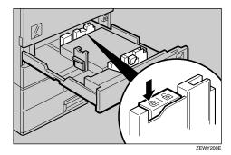
While pressing the release lever, adjust the back guide to the new paper size.
